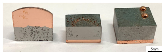
Figure 29. Samples from left to right: W_f/W -Cu rough interface before exposure, W_f/W -Cu flat interface after exposure, W_f/W -Cu rough interface after exposure - each sample is 12 mm wide.
