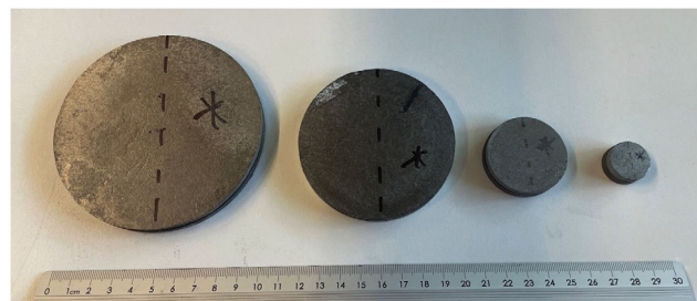
Figure 2. Four cylindrical stainless steel/ W_f/W test samples. From left to right: 105, 80, 40, and 20 mm.
