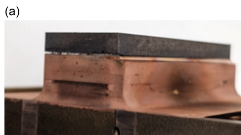
Visible gap between W_f/W composite tile and Cu interlayer after brazing..
