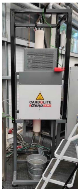
Figure 11. Quench test set up with argon inert gas heating and water quenchant.
